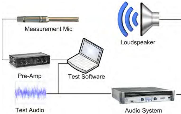
**Figure 2 Signal flow for testing time alignment**
