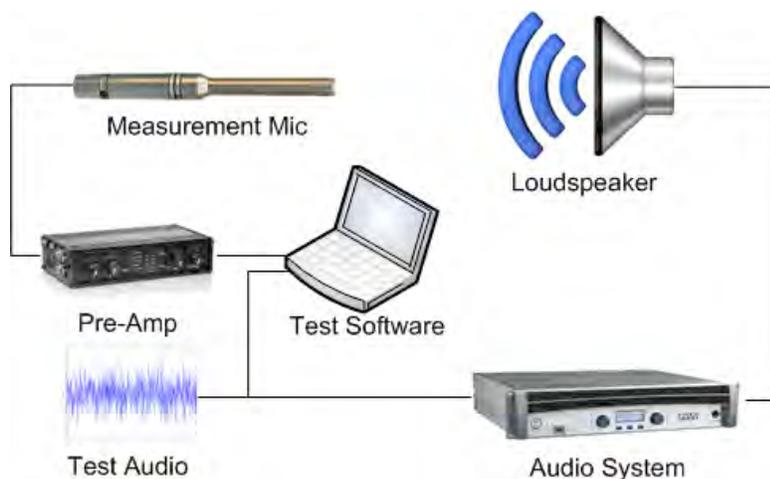
Figure 6 A typical setup for a dual channel test
