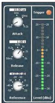
Figure 12 A peak program meter indicating 0 dBu
