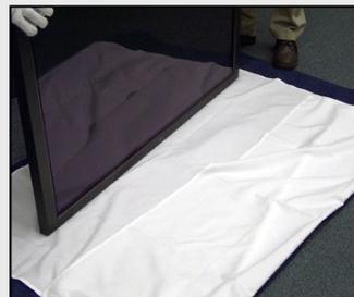
5. Carefully lay the flat panel display face down on a flat, clean shipping blanket. Make sure there are no tools or other obstacles under the blanket or damage will occur to the panel.
