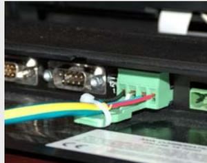
Captive screw connector and control panel
