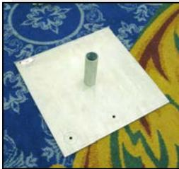
Floor bases are made of solid steel and are usually about 30 pounds (13.6 kilograms) each, 2 ft (0.6 m) on each side and 1/4 in. (0.63 cm) thick. There is a small hole in the center to which a stud is attached. This metal stud keeps the pole upright and prevents the set up from falling over.
