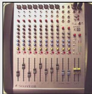
Here is an example of why a mixer is important... Assume you are using an audio system with two microphones that are connected to a mixer. During an event, one presenter is speaking very softly into her microphone on channel 1, and the other presenter is speaking very loudly into his microphone on channel 2. You can adjust the individual audio levels on each channel so the audience can hear both presenters comfortably. The outputs of each channel are combined and sent to the mixer's output.
