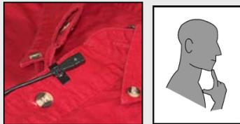
**Best practice:** Follow the “Forefinger and Thumb Rule” to place a lavalier microphone on a presenter. When placing the tip of the forefinger on the chin and the thumb toward the throat, the thumb’s position indicates the appropriate location where the microphone should be attached.
