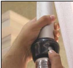
The hollow, aluminum poles have a metal pressure ring used to adjust the height of the pole. As you raise the pole, the pressure ring keeps it at the new adjusted height.
