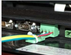
Captive screw connector and control panel
