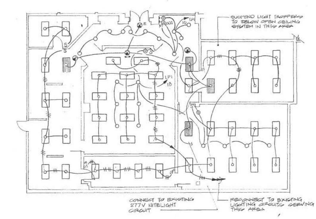
FIRST FLOOR PLAN - LIGHTING SCALE:1/8"=1'-0"
